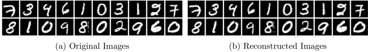
Figure 5.2: A network has been trained on each individual image to generate a corresponding resolution-independent encoding. Images were then reconstructed at the original resolution.
